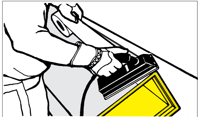
Fig. 4-4A. Apply heat with iron. Do not use a blowtorch; both heat and pressure are required for an effective bond. Complete the bond with a second pass of the iron.
