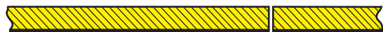
#SCO. Straight cutoff tool. May be used with #R1 to make the same cut as #7 tool.
