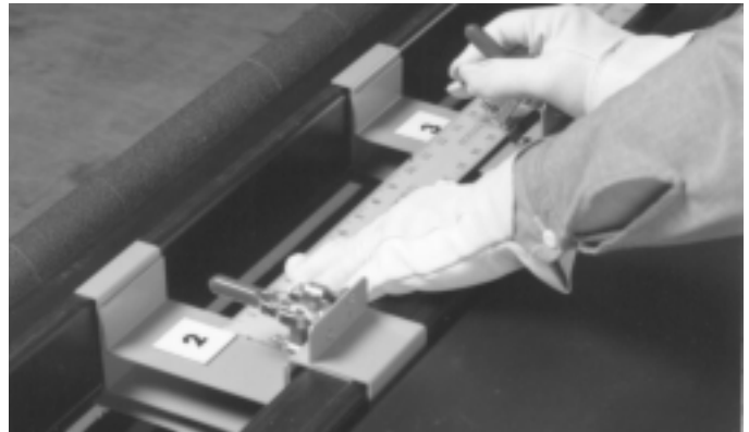
Fig. 2-9. Install tools in grooving machine according to machine manufacturer's instructions, board layout, and cutting plan (see pages 2-12 - 2-15), using either Standard or Preferred tooling set-up (see page 2-10).
