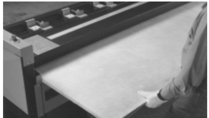
Fig. 2-10. Feed duct board into machine, female shiplap edge first, left hand edge firmly against guide, parallel to rollers. Turn on machine and guide board as friction rollers pick it up and pull it through the cutting tools.
