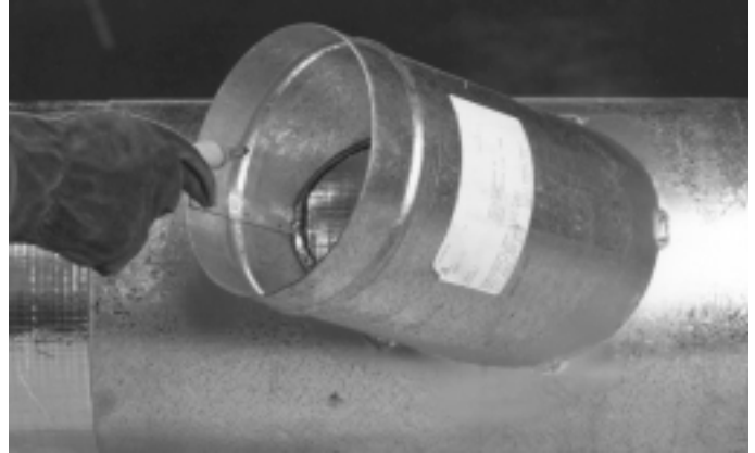
Fig. 7-6A. Marking hole for branch connection.
