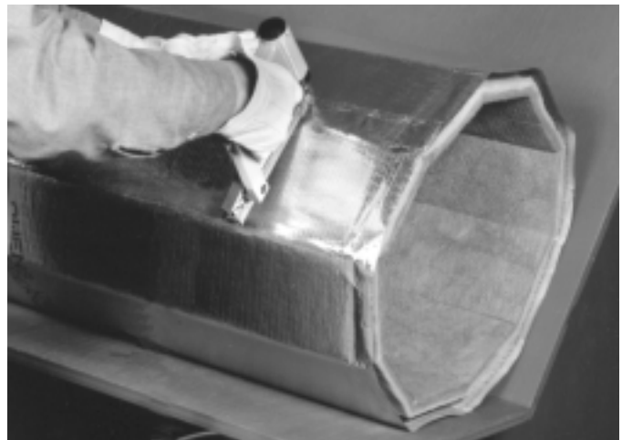
Fig. 3-34B. Stapling longitudinal joint of ten sided duct.
