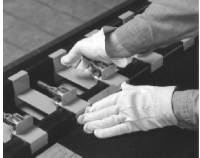
Fig. 3-31A. Duct board grooving machine set up for cutting ten-sided fibrous glass duct.
