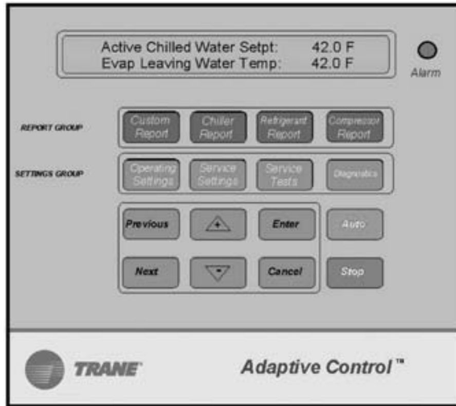
Figure 35 Operator Interface Adaptive Control
